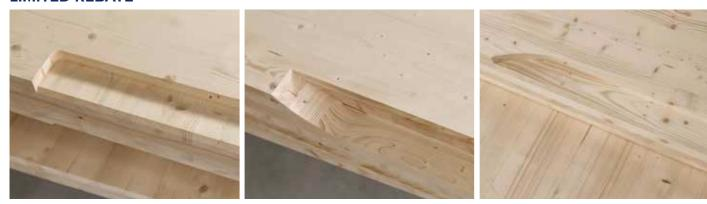
We create a limited rebate using the cylindrical mill cutter or end mill. Round shapes can also be created here depending on the tool used.
