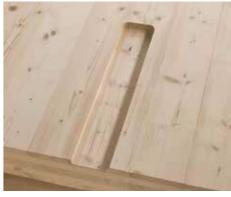
We use an end mill or cylindrical mill cutter to create slots – recesses with a limited depth – for example to inlay steps in a staircase or to mount steel brackets and connectors. These elements can also be rounded depending on the tool used.
