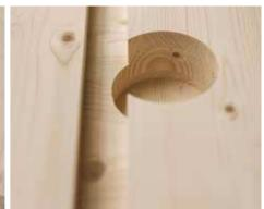
Holes can be drilled for cable ducting, sockets, as a pilot hole for subsequent screw connections, and other uses. We can use a 32 mm deep-hole drill to create electrical ducts inside visual-quality wood products.
